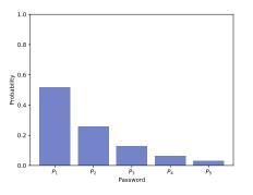
Figure 1: The simple, minimal example of a password probability distribution that we use to visualise different reselection modes in this section. Probability  $D(P_n)$  of password  $P_n$  is  $\frac{1}{2^n}$ .
