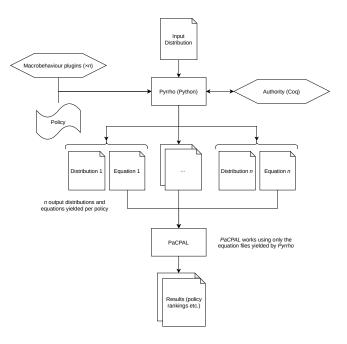
Figure 9: An overview of the function of Skeptic. Arrows indicate the direction of data flow.
